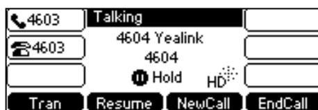
The line key LEDs on phone A slow flash green and phone B slow flash red when the shared line call is placed on hold.
