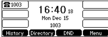
The idle screen displays the label of current account, time and date, and four soft keys.
