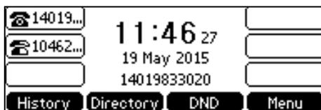
Any IP phone can be used to originate or receive calls on the bridged line. An incoming call to the BLA number can be presented to multiple phones in the group simultaneously. The incoming call can be answered on any IP phone of the group but not all.
