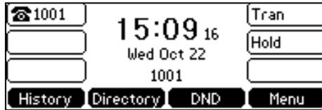
When you assign functionalities to line key 7-15, labels of the line key 6-10 are indicated on the second page, and labels of the line key 11-15 are indicated on the third page. The line key in the right bottom is used to switch pages.
