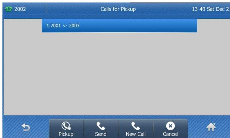
When there is an active call on the IP phone, you can transfer the active call to the monitored phone number directly by tapping the BLF key. The phone transfers the active call differently depending on the transfer mode via DSS key. For more information on performing call transfer, refer to [Call Transfer](#) on page 111.
