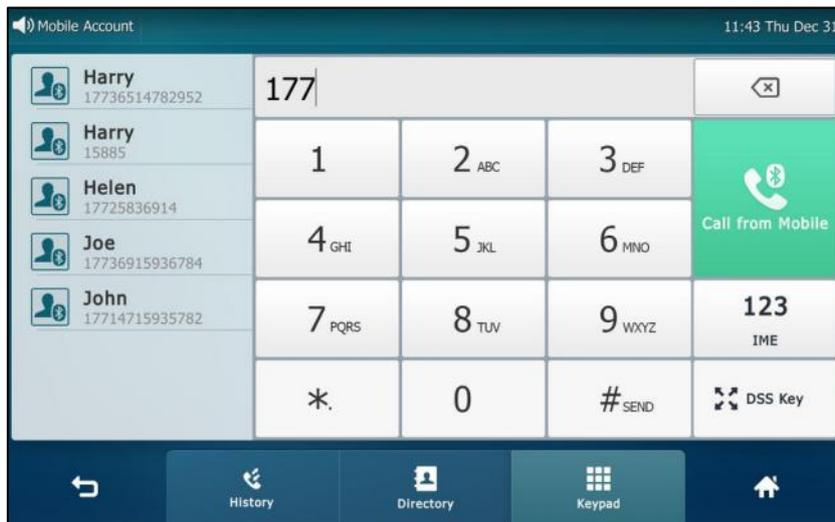
The outgoing call information will appear on both your IP phone and mobile phone screen. After the call is picked up, the audio goes through the IP phone, although the mobile phone screen also shows a connected call. You can hold, mute or end the call on the IP phone, and after you hold the call you can resume the call or place a new call.
