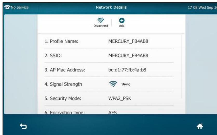
If the IP phone is being connected to a wireless network successfully, you can also tap **Wireless Status** to view the connected wireless network information.
